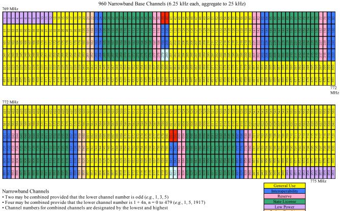
channel numbers separated by a hyphen, *e.g.*, "1-2" and "1-4". • Narrowband channels must maintain a data throughput efficiency of not less than 4.8 kbps for each 6.25 kHz of bandwidth
